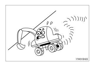
The engine angularity limits are 30 degree. Do not operate by more than the engine limits in any case.
